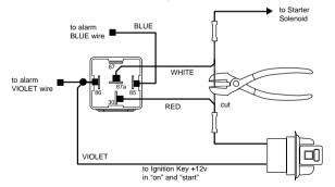
In this configuration, the vehicle's starter will be disabled only when the system is armed and alarming. If power to the system is lost or the system becomes disconnected, the vehicle will be able to start.
